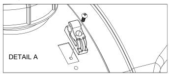
Locate the (2) clips and (2) phillips head screws from the parts bag.
